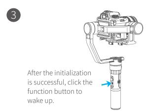
Note: if the initialization is not successful for a long time, long press the function button to turn off the gimbal, restar it and then initialize.
