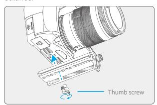
\*The screw is screwed into the threaded holes on the quick plate.
