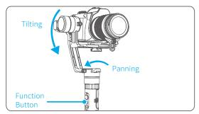
4. Pull the gimbal (which can be rotated more than one turn) to the rotation path you want to set, and then click the function button to record the end position.
