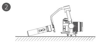
Place the gimbal on a flat surface. The gimbal will automatically initialize when it detects the non movement. The blue light will flash three times and initialization ends, otherwise, the initialization fails.
