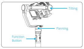
3. Set the gimbal start rotation position: pull the tilting axis or panning axis to the start position by hand, click the function button to record the start position.
